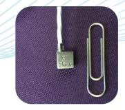
An Ultra-lightweight miniature triaxial vibration transducer comprising of three voltage output piezo-electric accelerometer elements mounted orthogonally within a titanium block. It makes use of the independent shear plate sensing elements, ensuring a rugged and repeatable triaxial measurement under the most extreme conditions. This design will outperform single element devices. The AT/08 uses high temperature piezo-ceramics as standard to ensure thermal stability.
