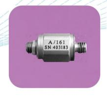
Developed for demanding applications requiring the measurement of high amplitude, short duration transient events such as pyrotechnic shock or high energy impacts, the A/16X range of stainless steel IEPE accelerometers have a range from 10,000g up to 50,000g
